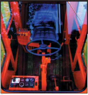
The picture above shows the operator's seat being positioned where he is completely protected from low-flying debris from almost every angle. He is also protected by an overhead guard made from 2" x 4" steel tubing.
