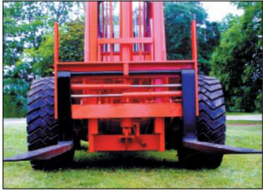
The DN4W Model shown above handles vehicles easily from the end. Notice the Power Adjustable Forks which hydraulically adjust from 60" wide to 14" wide with optional cab.
